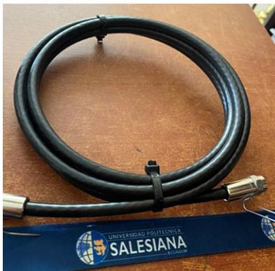
**Figura 4. Cable coaxial RG 58.**
