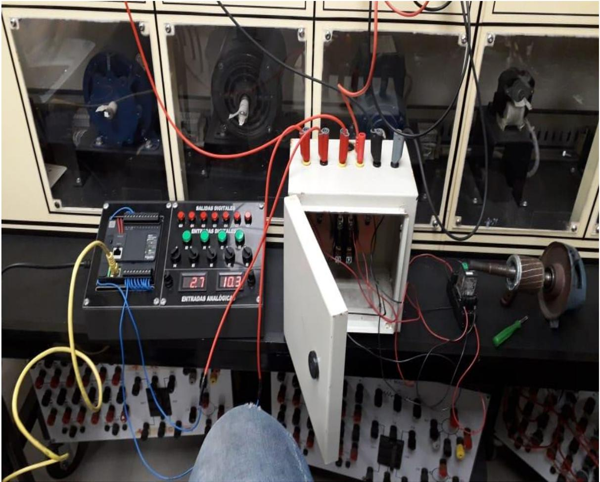
**FIGURA 69.** ACOPLAMIENTO DE RELÉ AL SISTEMA
