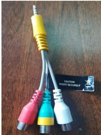
**Figura 20:** Cable conversor Jack 3.5mm a RCA
