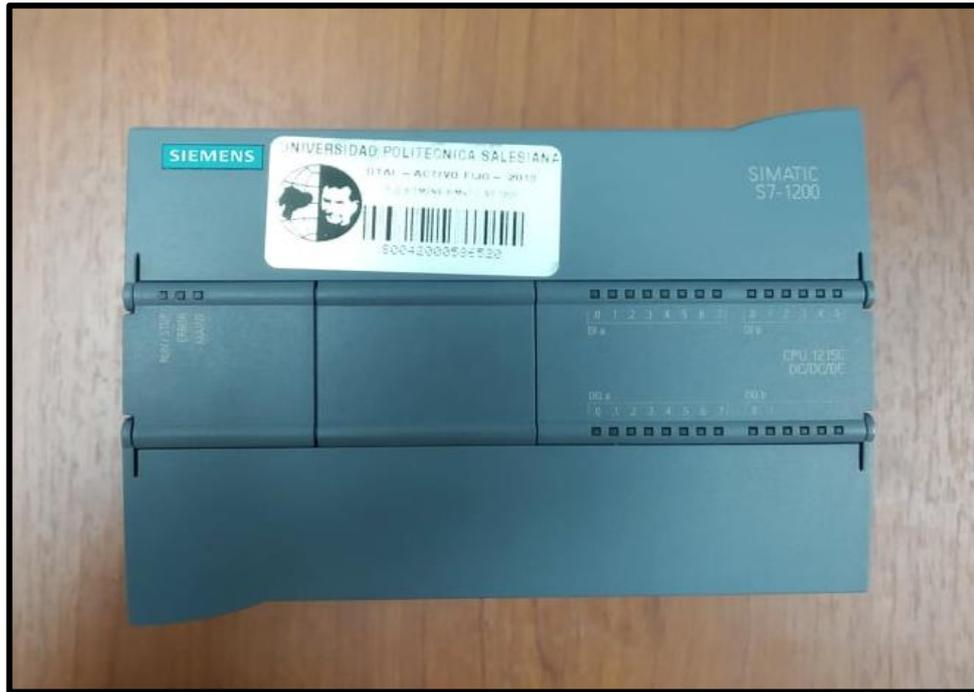
**Figura 53.** CPU 1215C DC/DC/DC Siemens.
