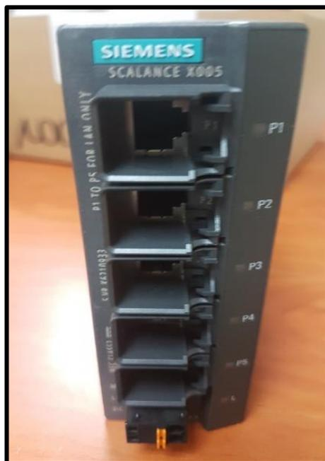
**Figura 55.** Switch Scalance X005 Siemens.
