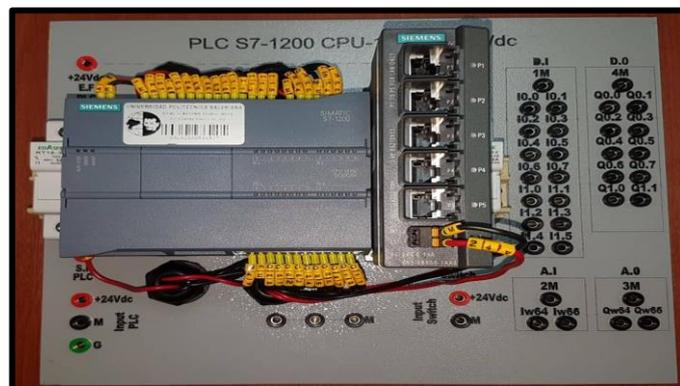
**Figura 65.** Lámina del PLC S7-1200 CPU 1215C Scalance X005.
