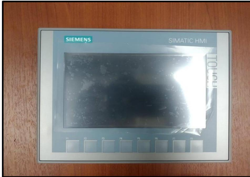
**Figura 57.** Simatic HMI KTP700 Siemens.
