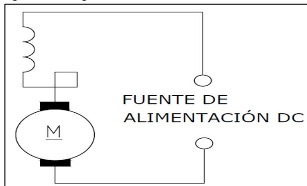
FIGURA 27: DIAGRAMA DE MOTOR EN SERIE CON INTERPOLOS
