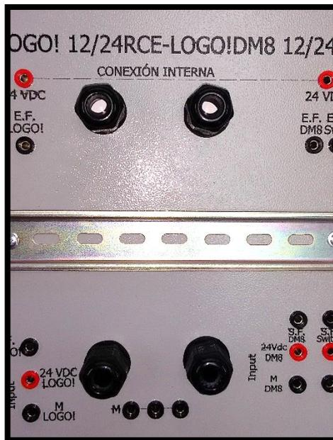
FIGURA 67: MONTAJE RIEL DIN, PRENSA ESTOPA Y BORNERAS.
