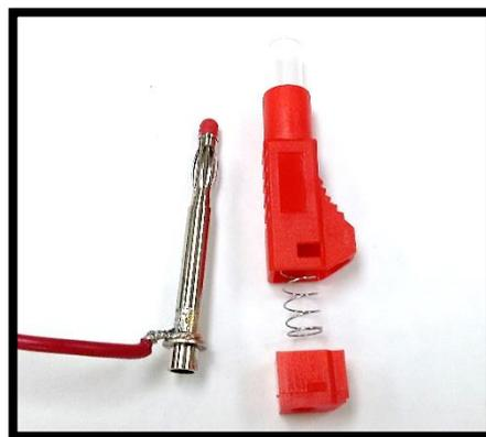
FIGURA 77: ENSAMBLAJE DE UN CONECTOR.
