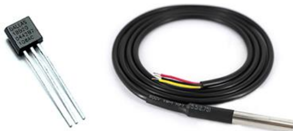
Figura 23: Sensor de temperatura ONE WIRE DS18B20 (DFRobot, 2008)
