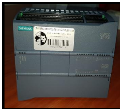
Figura 1. PLC S7-1200 CPU 1215C DC/DC/DC.
