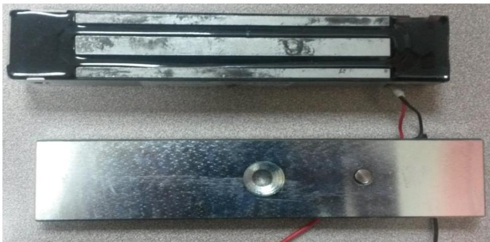
**Figura 19. Chapa Electromagnética (SECO-LARM U.S.A., Inc)**
