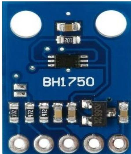
**Figura 12. Sensor de Luz BH1750 (Naylamp Mechatronics)**
