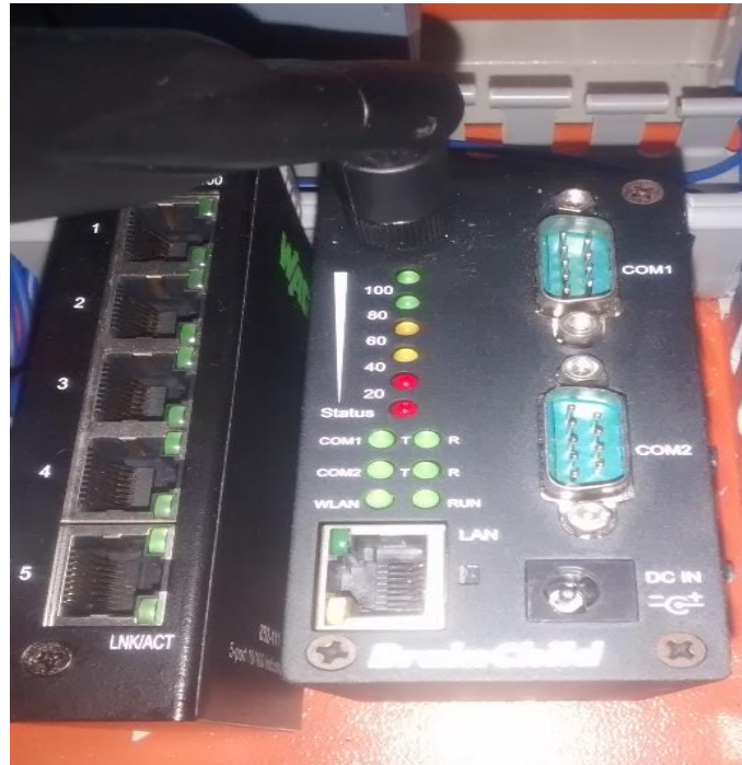
Figura 48. Antena alto alcance SW5502 (BrainChild, 2018)
