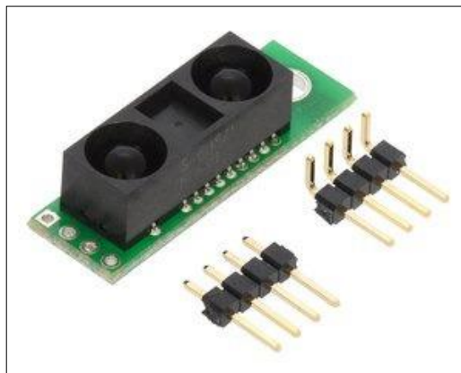
Figura 12: Sensor de distancia GP2Y0A60SZ (Pololu Corporation , 2018)
