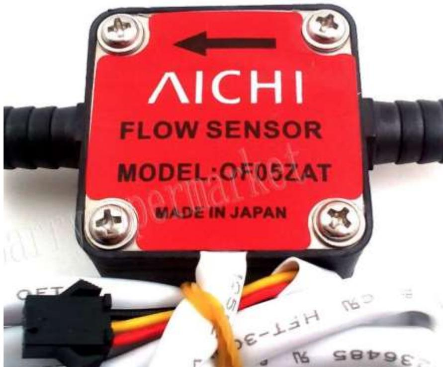
*Figura 4 Flow Sensor Fuel (Autor)*
