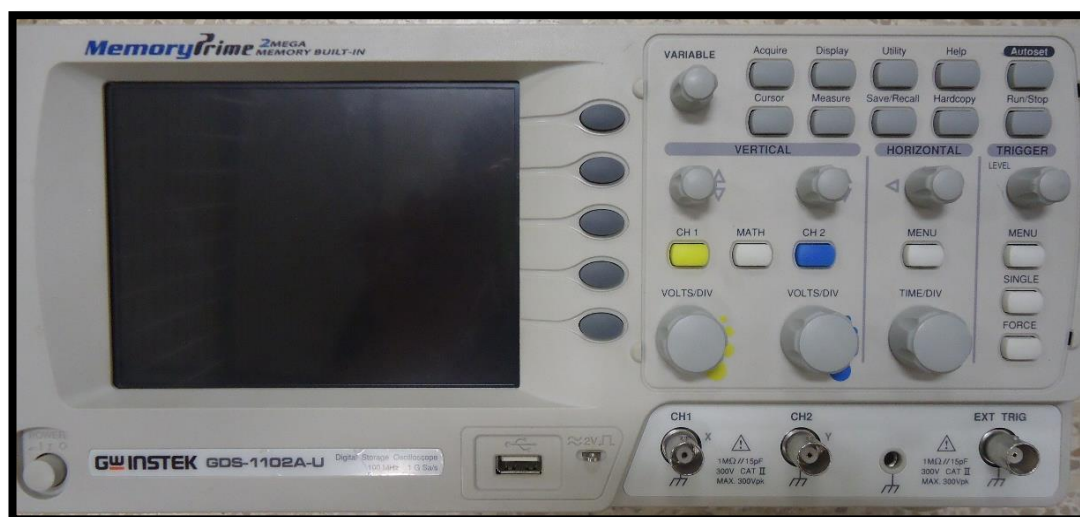
FIGURA 42: OSCILOSCOPIO GW INSTEK GDS-1102A-U [36]
