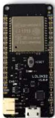
Figura 3.22 Placa Lolin32 de WEMOS Electronics [60]
