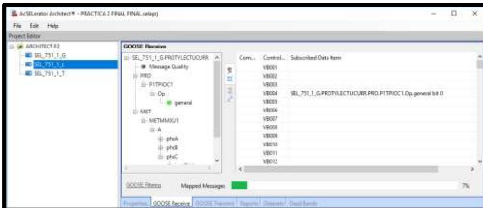
FIGURA 109: AJUSTE DE RECEPTOR GOOSE – VALORES BOOLEANOS
