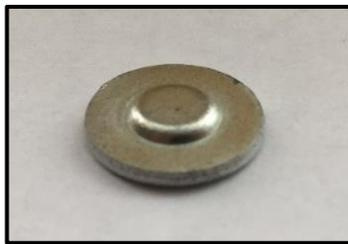
Figura 71. Arandela defectuosa vista inferior
