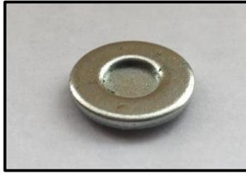
Figura 70. Arandela defectuosa vista superior
