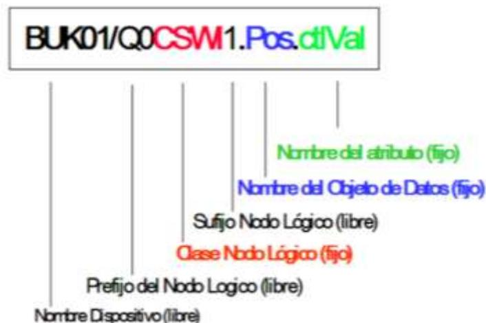
FIGURA 32: ESTRUCTURA GENERAL DE UN DATO
