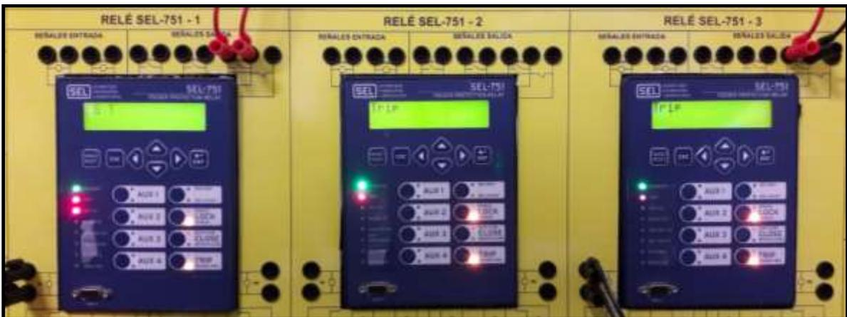
FIGURA 188: FALLA EN LA BARRA – 50P – APLICANDO METODOLOGÍA GOOSE
