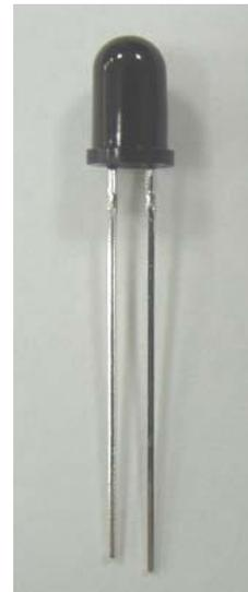
5  $\phi$  plastic package. Due to its black epoxy the device is sensitive to infrared radiation.
