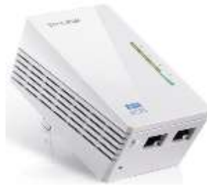
Figura 3: Extensor Powerline WiFi AV500 a 300 Mbps TL-WPA4220
