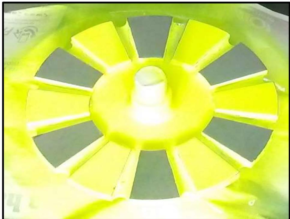
*Figura 12.* Rotor inductor
