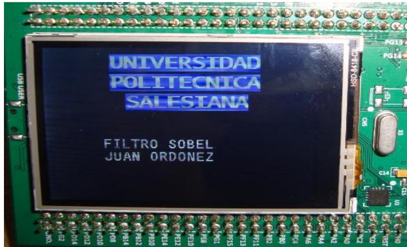
Figura 8. Pantalla LCD 2.4" QVGA TFT
