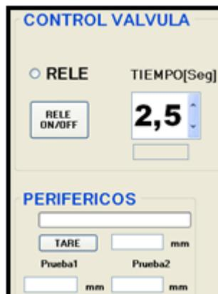
The screenshot shows a software interface titled 'CONTROL VALVULA' (VALVE CONTROL). It features a 'RELE' (RELAY) control section with a radio button and a 'TIEMPO[Seg]' (TIME[Sec]) section with a digital display showing '2,5' and a 'RELE ON/OFF' button. Below is a 'PERIFERICOS' (PERIPHERALS) section with a 'TARE' button and two input fields for 'Prueba1' and 'Prueba2', both labeled 'mm'.
