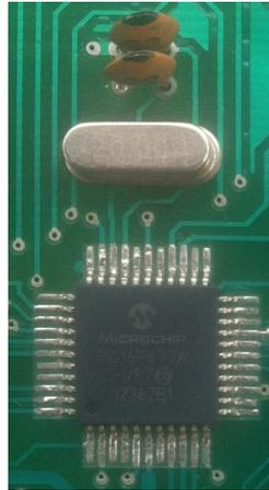
**Figura 3.21:** Microcontrolador principal PIC 16F877A-QFT
