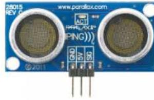
**Figura 2.39:** Sensor Ping de Parallax
