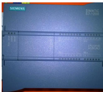
Figura 71: PLC SIMATIC S7-1200 / CPU 1214C
