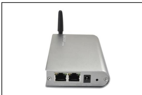
**Figura 2.24. Gateway SIP GSM DWG2000-1G**
