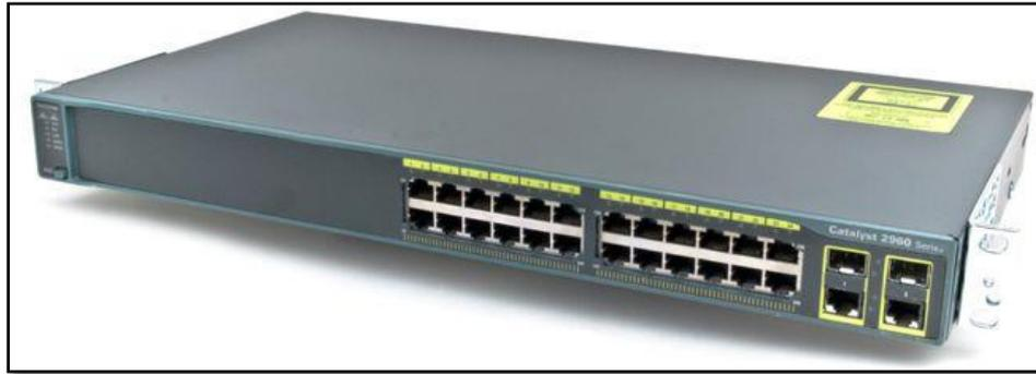
**Figura 2.26. Switch Cisco Catalyst 2960**
