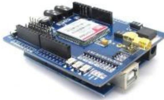
IComsat is a GSM/GPRS shield for Arduino and based on the SIM900 Quad-band GSM/GPRS module. It is controlled via AT commands (GSM 07.07 ,07.05 and SIMCOM enhanced AT Commands), and fully compatible with Arduino / Iteaduno and Mega.
