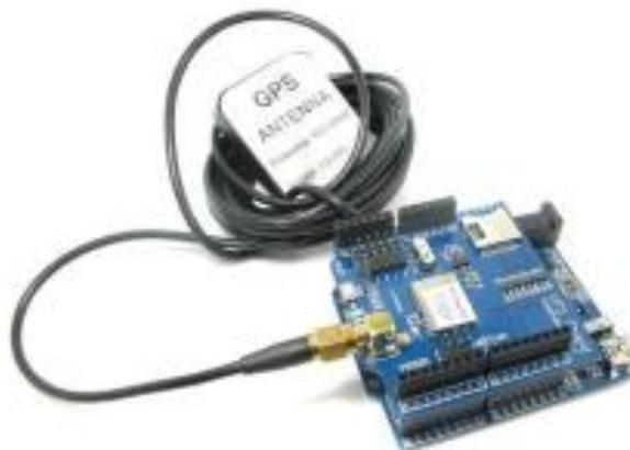
Arduino GPS shield is a GPS module breadout board designed for Global Positioning System receiver with SD interface. It is easy to use for recording the position data into SD card. 5V/3.3V compatible operation voltage level make it compatible with Arduino boards, leaf maple, IFlat32 and other arduino compatible boards.
