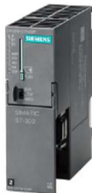
SIMATIC S7-300 CPU 315-2 PN/DP, CENTRAL PROCESSING UNIT WITH 384 KBYTE WORKING MEMORY, 1. INTERFACE MPI/DP 12MBIT/S, 2. INTERFACE ETHERNET PROFINET, WITH 2 PORT SWITCH, MICRO MEMORY CARD NECESSARY
