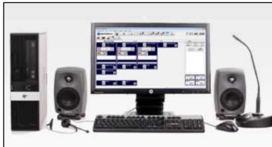
*Figura 3.3 Consola De Despacho IP MCC 7500.
