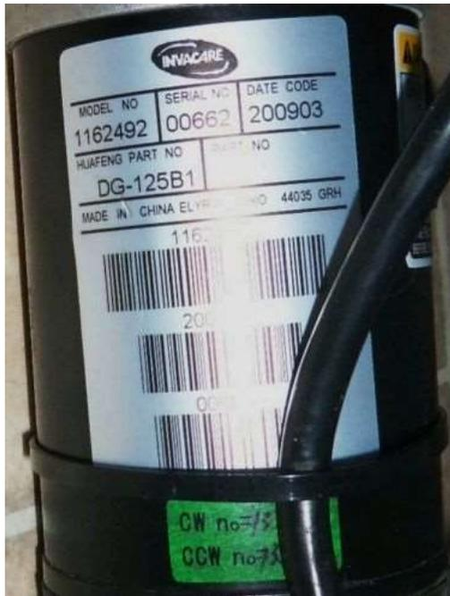
COMPLETE ELECTRIC WHEELCHAIR ROBOTICS drive system 24volt features HIGH TORQUE geared motors with electromagnetic disk brakes made by Invacare, these motors are high torque 24 volts DC, 50NM stall torque! & 110 RPM at the output shaft the output shafts are 45mm long & 17mm dia these are very high quality motor units with aluminum gear box cases sealed & fully ball raced
