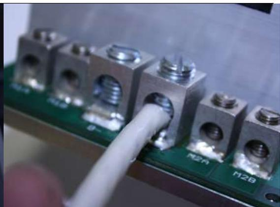
**Step 4:** Turn the top screw clockwise until you encounter resistance, then tighten the screw firmly. Pull on the wire gently to ensure that it is secured.
