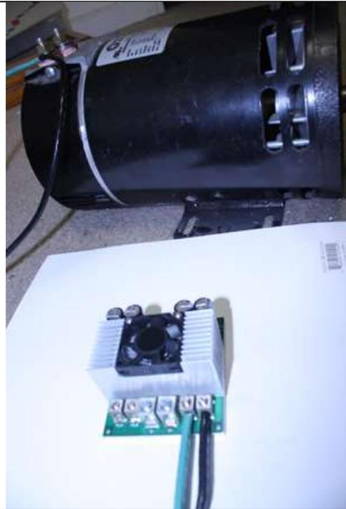
The motors connect to terminals M1A/B and M2A/B
