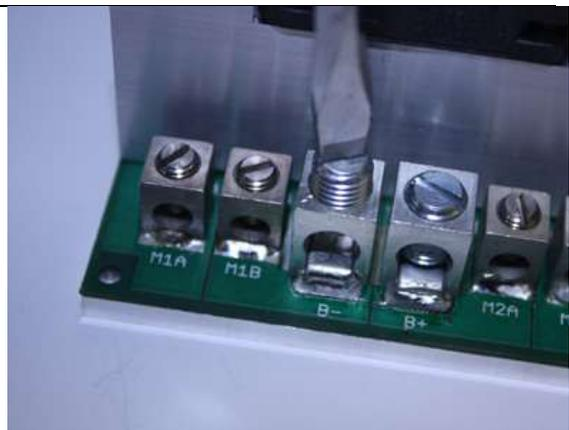
**Step 2:** With a medium sized screwdriver, turn the top screw counter-clockwise until there is enough clearance to fit the wire.
