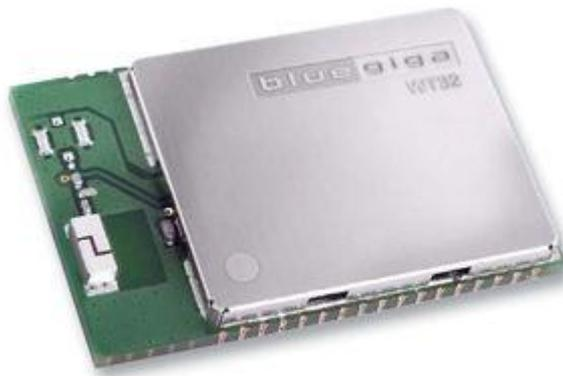
**Figura 2.7:** Módulo Bluetooth WT32 A AI3.
