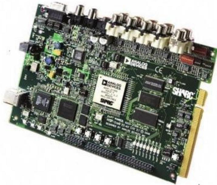
**Figura 2.13:** ANALOG DEVICES - ADZS-21369-EZLITE - ADSP-21369, VISUALDSP++, EVAL KIT
