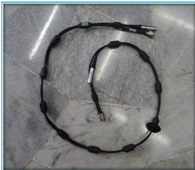
**Figura 50. Cable conector del SRM – 3000 a la Antena Triaxial**
