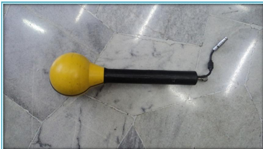
**Figura 48. Antena Triaxial SRM – 3000**
