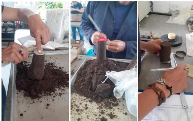
**Figura 4.5:** Ensayo triaxial (CU)
