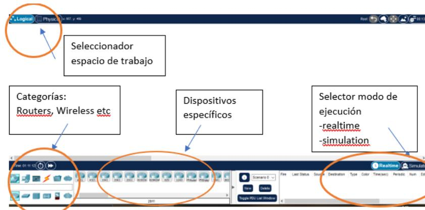
Figura 1: Pantalla principal Cisco (Cisco Packet Tracer, 2024)
