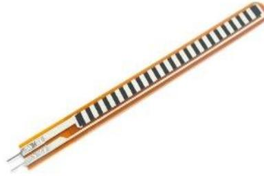
Fig. 15. Sensor Flex (Naylamp Mechatronics, 2021)
