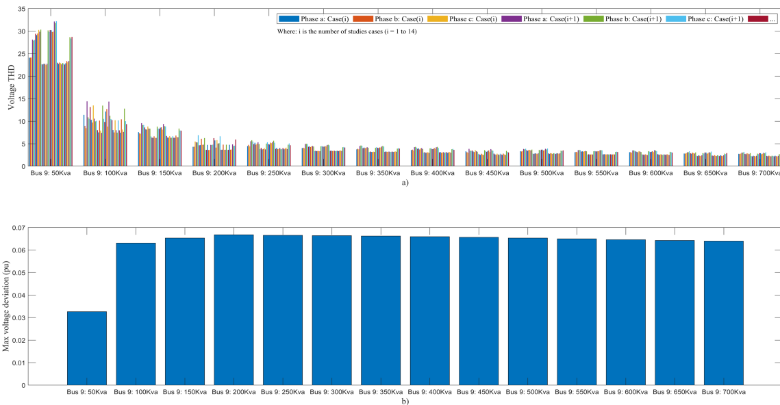
Figure 3.7: (a) THD per bus in maximum demand with compensation in bus 9 and (b) Maximum voltage deviation with compensation in bus 9 without considering the THD as an objective criterion.
