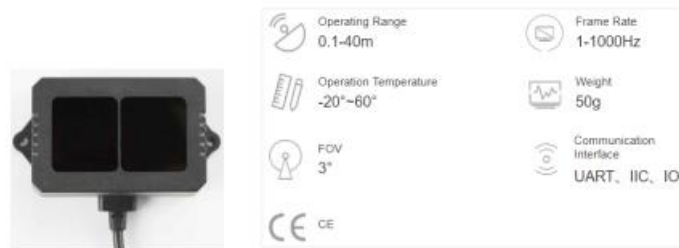
Figura 17 :LIDAR TF02-Pro
