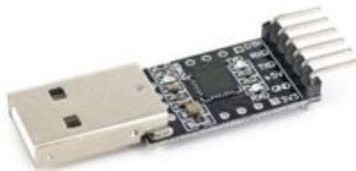
Figura 14. Módulo CP2102 conversor USB a serial [29]
