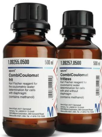
**Nota:** La grafica representa el reactivo Karl Fisher, la que utilizan en los laboratorios para realizar las pruebas aplicando la Normativa ASTM D-1744, adaptado de ([https://www.merckmillipore.com/INTL/en/product/CombiCoulomat-fritless,MDA\\_CHEM-109257?ReferrerURL=https%3A%2F%2Fwww.google.com%2F](https://www.merckmillipore.com/INTL/en/product/CombiCoulomat-fritless,MDA_CHEM-109257?ReferrerURL=https%3A%2F%2Fwww.google.com%2F))
