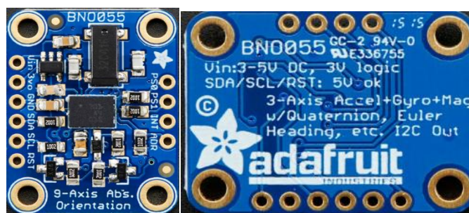
Figura.2.10 Sensor 9-DOF, BNO055
