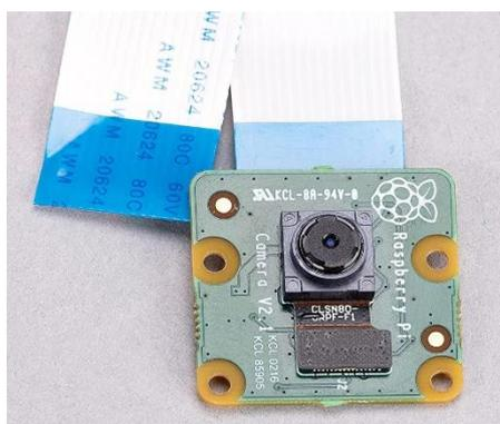
Fig. 16 Raspberry Pi Camera Module V2 8MP [13]
