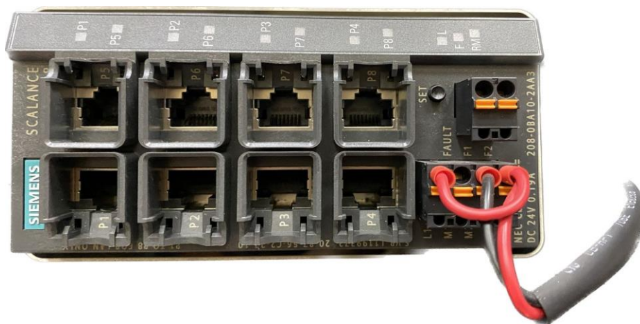
Figura 3.2: SIMATIC Ethernet Switch SCALANCE X208
