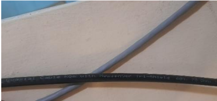
Figura 47. Cable coaxial RG6 de 75ohms.
