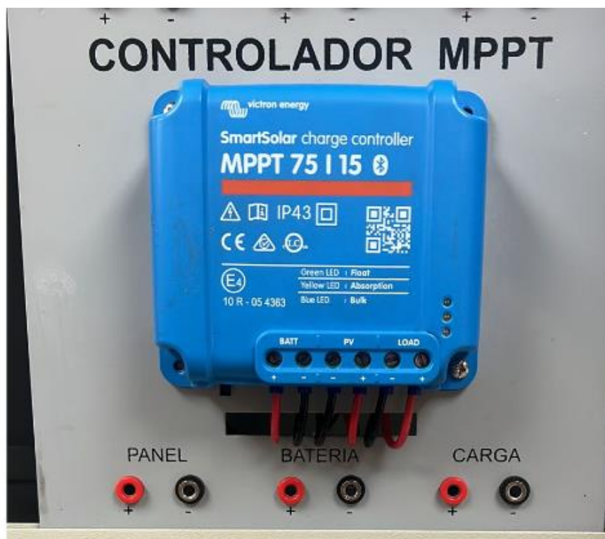
FIGURA. 18 CONTROLADOR MPPT (VICTRON ENERGY) (AUTOR)
