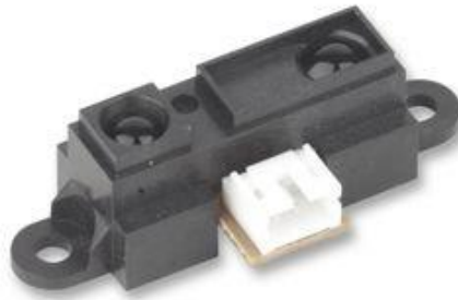
Figura 3.4: Sensor SHARP infrarrojo 4 a 30[cm]
