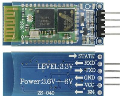
Figura 2.8: Módulo bluetooth HC-05. [Haq et al., 2021]
