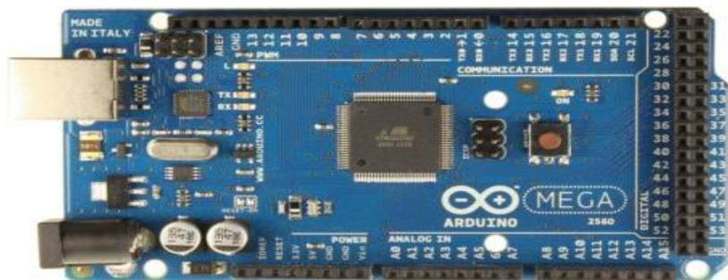
Figura 11 Arduino mega 2560 [27].
