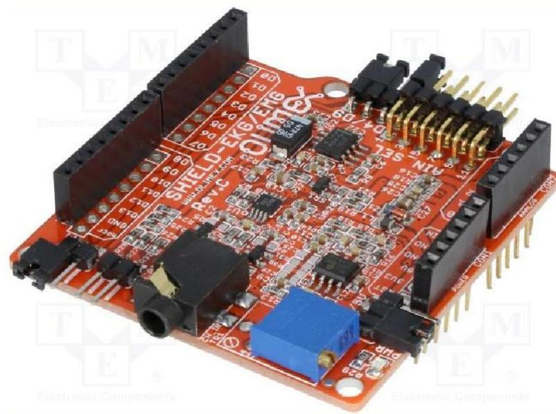
Figura 8 Shield-Ekg-Emg (Olimex, 2021)
