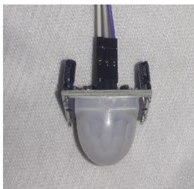
Figura 4. Sensor PIR HC-SR501.
