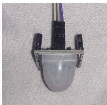
Figura4. Sensor PIR HC-SR501.
