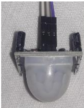
Figura 3. Sensor PIR HC-SR501.
