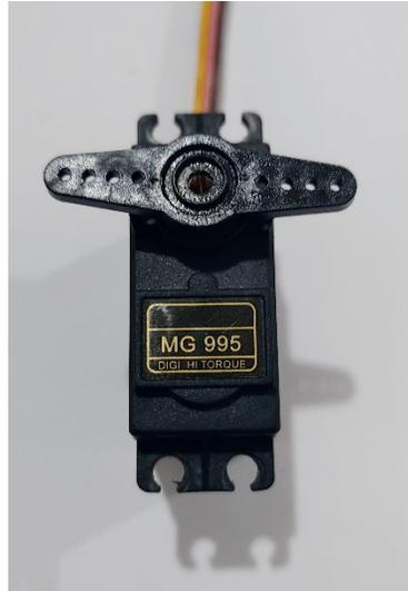
**Figura 3.31** Servomotor MG 995 15Kg/N.cm
